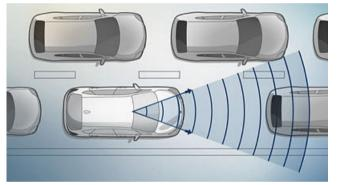
□ The **Traffic jam assistant**<sup>2</sup> controls the speed of the car and distance from the vehicle ahead in dense traffic on motorways at speeds of up to 60 km/h and provides steering assistance.
