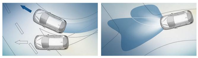
Dynamic Stability Control (DSC) constantly assesses the vehicle's movements and optimises directional stability and traction.
