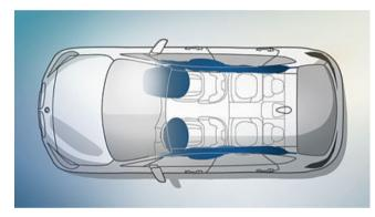
Airbags for the driver and front passenger, head airbags as well as side airbags integrated into the front seat backrests provide strategic protection.
